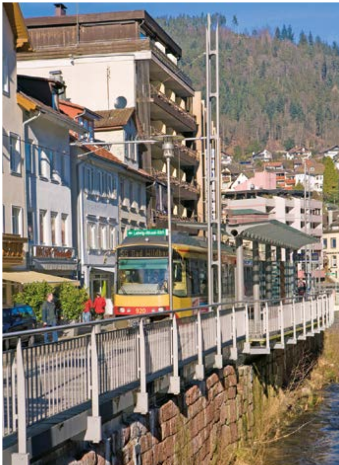
Enz Valley Railway: TramTrain on a street-running tramway section at Bad Wildbad.
