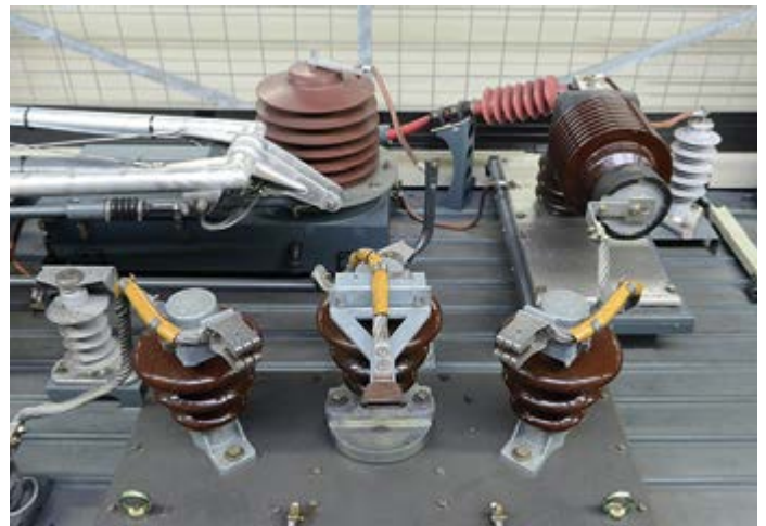
Current system selection relay on the roof of the TramTrain.
